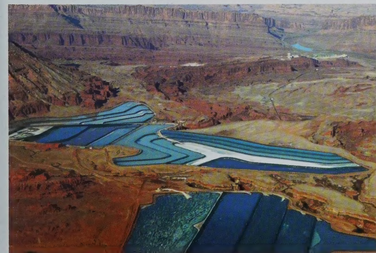
Intrepid Potash's solar evaporation ponds near Moab. The blue color is caused by dye added to the brine to increase evaporation. The dry potash is harvested and hauled for processing at the plant located in the upper-right part of the image. Photo credit: Intrepid Potash, Inc.
